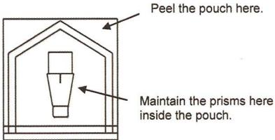
3. Place the separation prisms on the holder of the tonometer (the mark (indent) on the prism allows a clear positioning on the prisms holder ; align the mark on the prisms with the mark on the holder).
